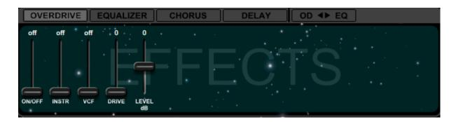
At lower levels, you can use this effect to create sounds that emulate the warmth and breakup of a tube amplifier. At higher levels you can create some quite grinding distortion sounds.
