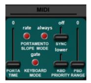
The parameters in this block are relevant only if the FI is being played using its MIDI IN port or if it is being synchronized to a MIDI clock signal via the MIDI IN port.
