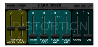
The Distortion Block applies distortion to the original instrument signal and to the three transposed voices generated by the Harmonizer.<sup>8</sup> VOICE1 is fixed at 1 octave above the input signal, whereas the transpositions of VOICE2 and VOICE3 are variable.
