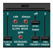
The parameters in this block are relevant only if the FI is being played using its MIDI IN port or if it is being synchronized to a MIDI clock signal via the MIDI IN port.
