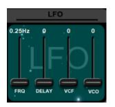
The FI has a dedicated Low Frequency Oscillator (LFO) for modulating the cutoff frequency of the VCF and the pitch of the VCOs. This can be used to create pitch vibrato and filter "wobbles".
