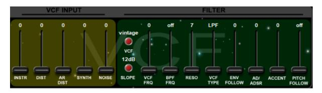
The Voltage-Controlled Filter (VCF) is one of the most important sound-shaping tools in a synthesizer. Basically it removes certain frequencies from a sound, thus altering its harmonic content. Depending on the type of filter used, the frequencies *above*, *below* or *at* a specified "cutoff" frequency are removed. This cutoff frequency can be modulated dynamically from different sources (e.g. an envelope), thus creating sounds which evolve over time.
