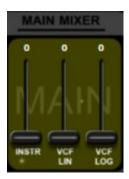
This is a simple two-channel audio mixer situated before the final output to the effect section.
