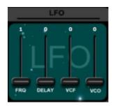
The FI has a dedicated Low Frequency Oscillator (LFO) for modulating the cutoff frequency of the VCF and the pitch of the VCOs. This can be used to create pitch vibrato and filter "wobbles".
