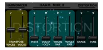
The Distortion block applies distortion to the original instrument signal and to the three transposed voices generated by the Harmonizer.<sup>2</sup> VOICE1 is fixed at 1 octave above the input signal, whereas the transpositions of VOICE2 and VOICE3 are variable.
