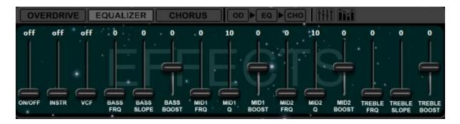
The Equalizer consists of a bass shelf tone control, two parametric band equalizer stages, and a treble shelf tone control.
