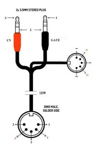
Connect the CV cable (red plug) to the 1V/Oct pitch input of your synthesizer. Connect the Gate cable (black plug) to the gate input of your synthesizer. Note that some synthesizers have separate gate inputs for the VCA and VCF envelopes, in which case you will need to use a hub or splitter cable attached to the gate cable to send the signal to both destinations.
