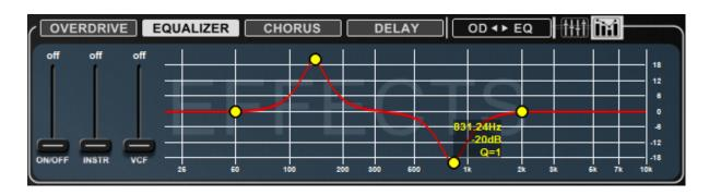
This block contains four effects: <u>Overdrive</u>, <u>Equalizer (EQ)</u>, <u>Chorus</u> and <u>Delay</u>. Up to three of the effects can be used simultaneously, though <u>Chorus and Delay cannot be used</u> <u>together</u>. Chorus or Delay is fixed at the end of the chain but the order of the other two can be changed at will. The effects are fed by the INSTR and VCF outputs from the Main Mixer.
