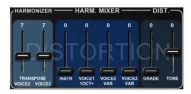
The Distortion Block applies distortion to the original instrument signal and to the three transposed voices generated by the Harmonizer.<sup>16</sup> VOICE1 is fixed at 1 octave above the input signal, whereas the transpositions of VOICE2 and VOICE3 are variable.
